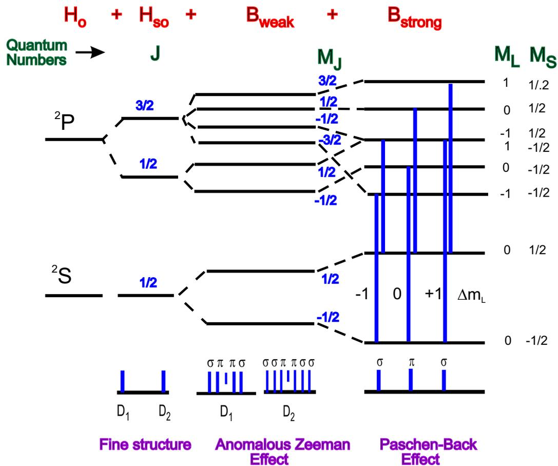
Figure 32: Diagram showing splitting of Na 3p-levels from zero field, through weak to strong field showing change from Anomalous Zeeman to Paschen-Back effect.
