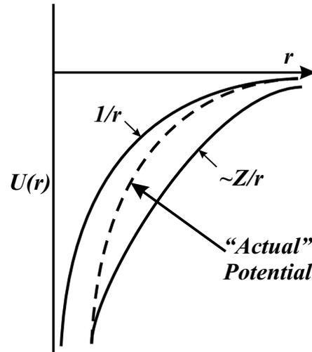
Figure 5: “Actual” potential experienced by an electron behaves like  $1/r$  at large  $r$  and  $Z/r$  for small  $r$ . The intermediate  $r$  case is somewhere between the two.
