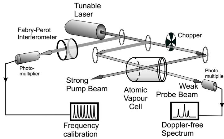
Figure 41: Saturated absorption spectroscopy. A beam from a tunable laser is split into a strong (pump) beam and a weak (probe) beam which intersect at a small angle in the absorbing gas. When the frequency of the light is resonant with an atomic transition the absorption of the weak probe beam is reduced owing to saturation by the pump. The chopper modulates the pump beam so that the saturation effect is detected above the noise on the detector of the probe beam.
