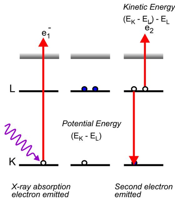
Figure 39: Ejection of a second electron following ejection from an inner shell, resulting from excess energy given to an electron when one electron in the same shell falls to a lower vacancy.
