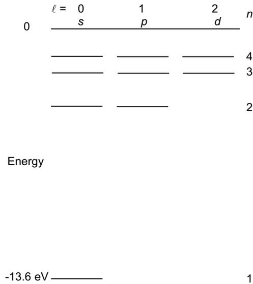
Figure 7: Energy level structure of hydrogen, illustrating how the bound state energy depends on  $n$  but not  $l$ .
