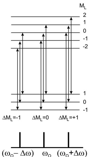
Figure 25: Normal Zeeman effect gives the normal Lorentz triplet due to selection rules  $\Delta M_L = 0, \pm 1$  and splitting of all levels into equally spaced sub-levels  $M_L$ .
