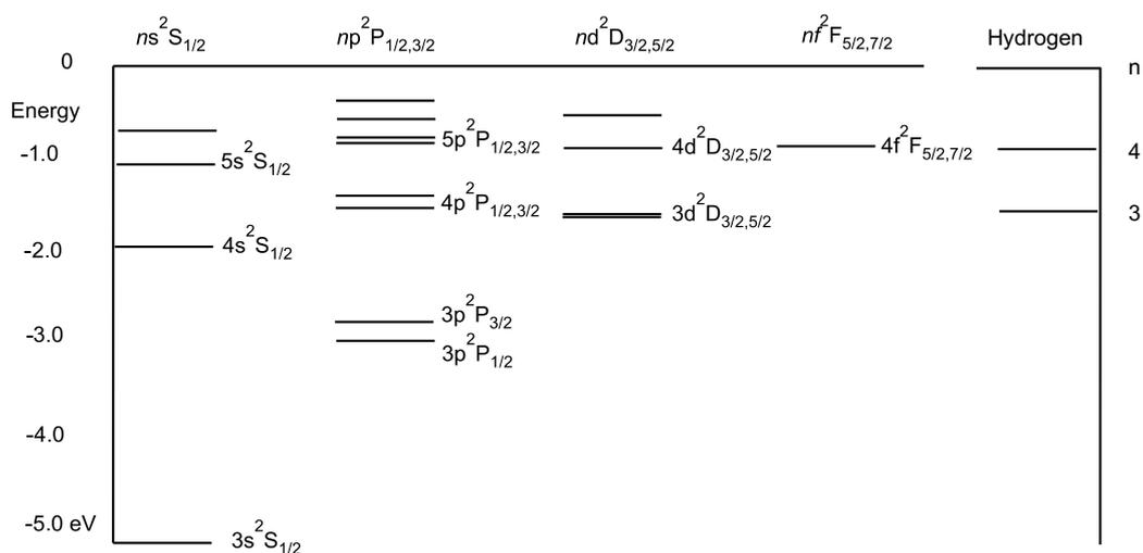
Figure 16: Na energy level diagram showing fine structure (spin-orbit splitting) greatly exaggerated. Note that the difference between energy levels the same  $n$  but of increasing  $l$  become smaller as they approach the hydrogenic energy level for the corresponding  $n$ . Note also that the difference between energy levels of the same  $n$  but different  $l$  becomes smaller with increasing  $n$ .
