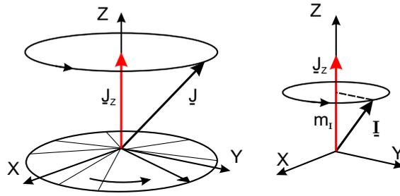
Figure 35: Effect of strong field on hfs: the total electronic angular momentum  $\underline{J}$  precesses rapidly around  $\underline{B}_{\text{ext}}$  ( $z$ -axis). As a result the nuclear spin  $\underline{I}$  can follow only the time averaged projection of  $\underline{J}$  on the  $z$ -axis.
