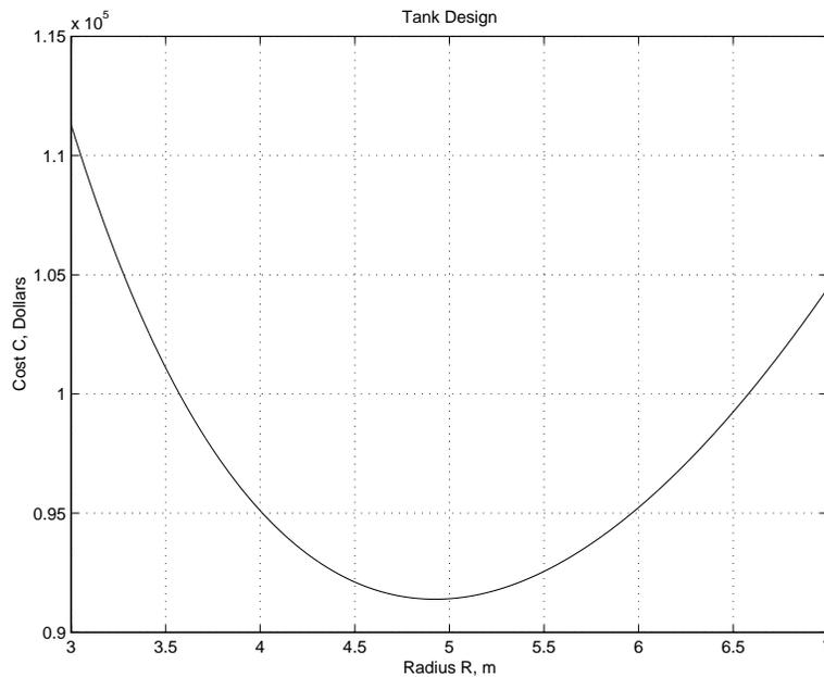
Figure 7.3: Tank design problem: cost versus radius
