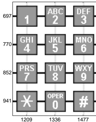
The tone generated by the button in position  $(k, j)$  is obtained by superimposing the two fundamental tones with frequencies  $fr(k)$  and  $fc(j)$ .
