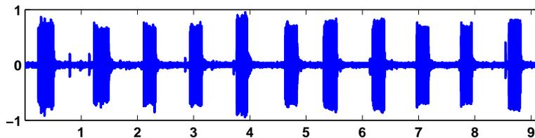
**Figure 8.2.** *Recording of an 11-digit telephone number*
